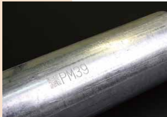
Mark 2D code on pipe.
