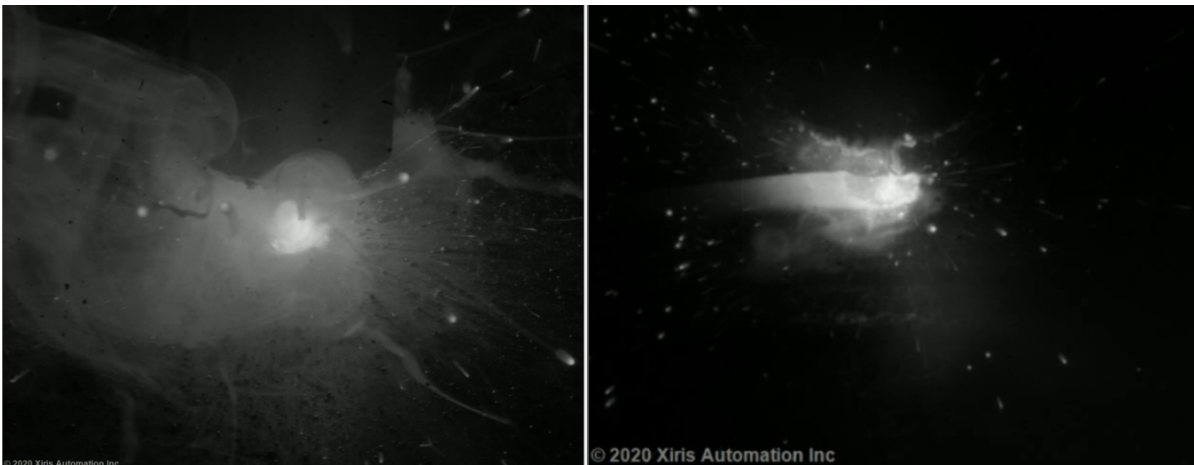
Figure 5- Comparative images showing the same welding process in visible and in SWIR using a XIR-1800 Thermal Camera (Source: Xiris)
