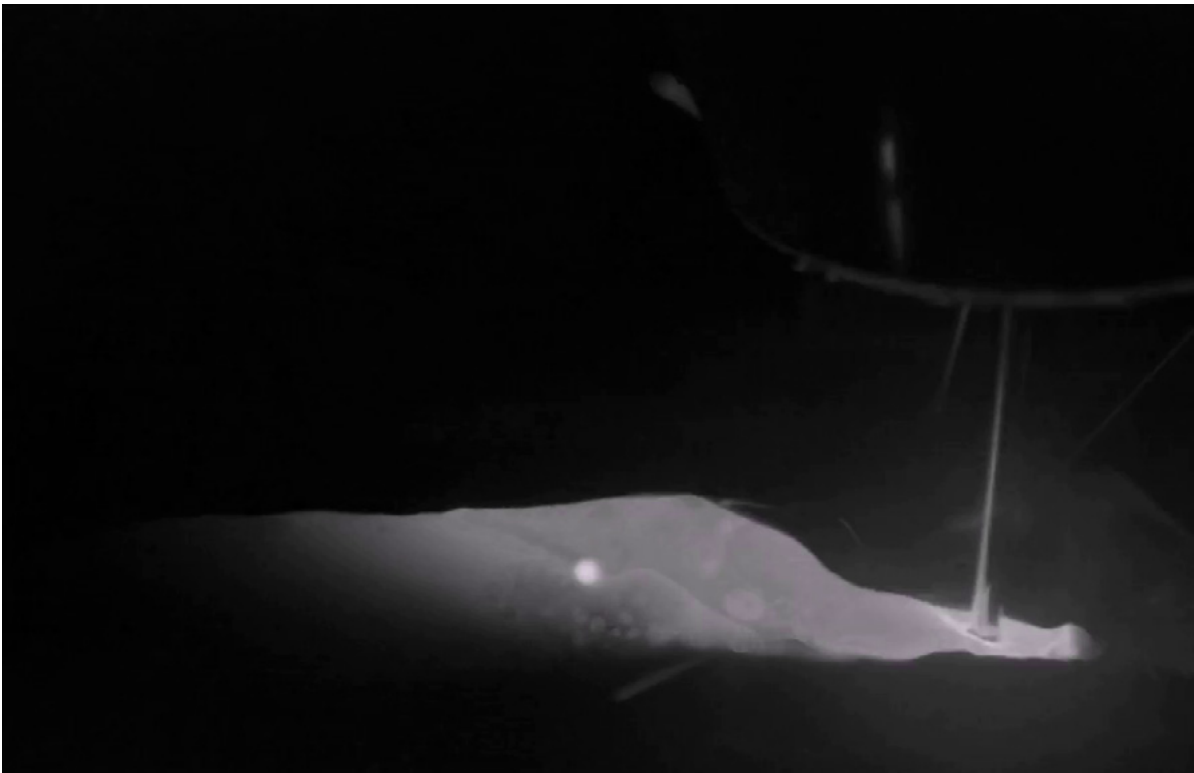
A video showing metal transfer in a Pulsed GMAW Process
