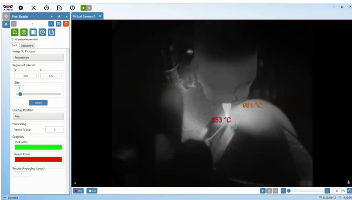
A photo of GTAW welding process with the Pixel Reader measurement tool
