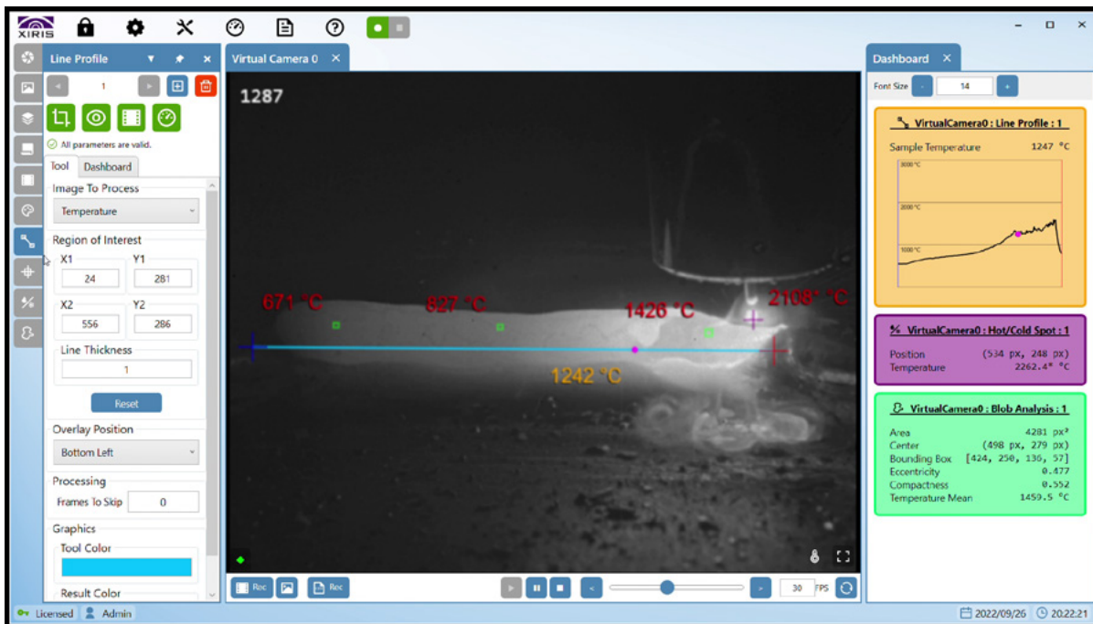
A video of a GMAW welding process with Line Profile and Pixel Reader measurement tools
