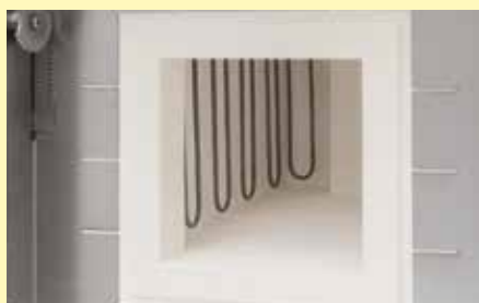
High-temperature heating in furnace chamber
