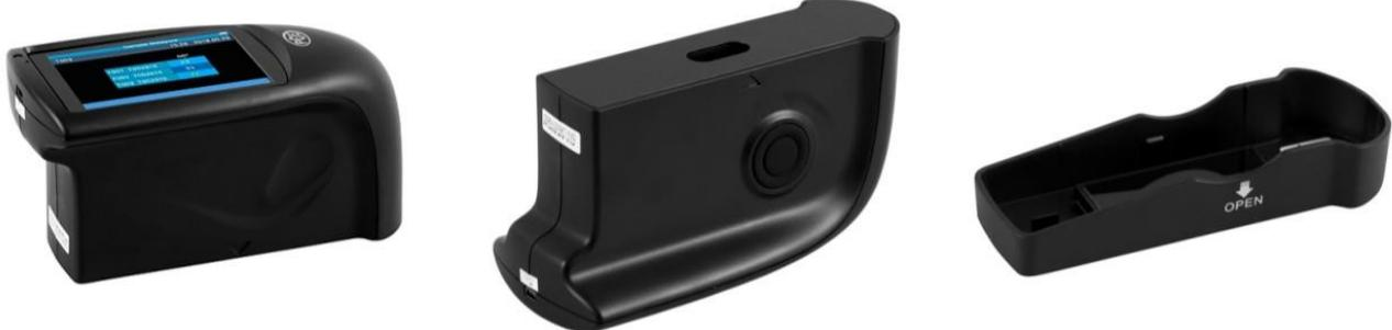
**Gloss Meter PCE-GM 60Plus-ICA for non-stationary use / Measurement up to 200 gloss points / 60° Measurement geometry/ 3.5" TFT display / short measuring time of 0.5 seconds**
