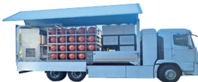
L,P ( 70 BAR )Filling Station
