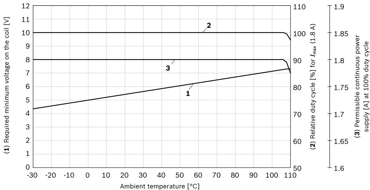
▼ **Control pressure 18 and 30 bar, 24 V ( $R_{\text{nom}} = 12 \Omega$ ;  $I_{\text{max}} = 0.8 \text{ A}$ )**
