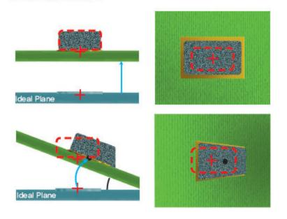
When a PCB moves up or down relative to the ideal plane, the size of an object, from the camera's viewpoint, will appear to be either larger or smaller, respectively.
