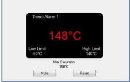
**Therm-Alarm**® prevents temperatures from exceeding user-defined limits.
