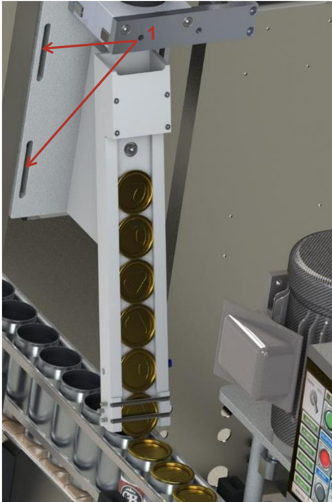
Figure 23 Setting bolts to adjust can lid dispenser height
