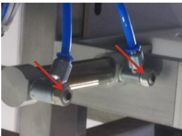
Figure 28 Adjusting air flow control screws on seam station air cylinder
