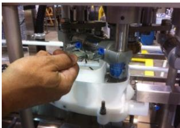
Figure 28 Adjusting air flow control screws on seam station air cylinder
