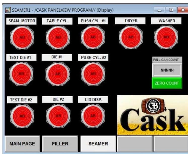
Figure 9 HMI Screen – Seamer page screenshot
