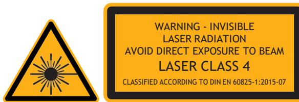
Figure 4.5.: Warning labels for laser radiation and laser class
