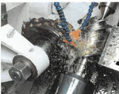
Milling process of rotor
