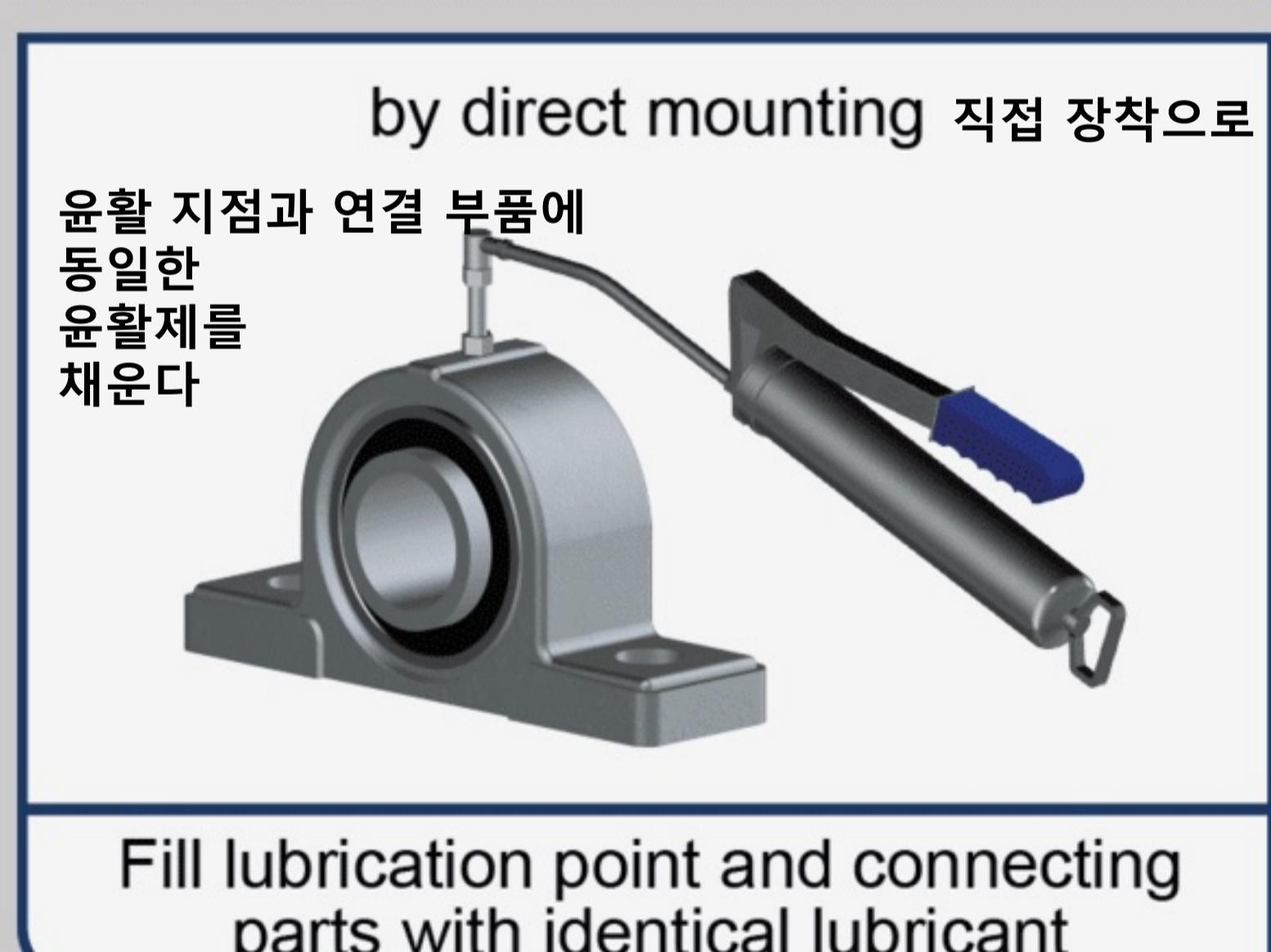
Fill lubrication point and connecting parts with identical lubricant
