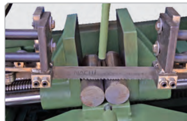
Improved blade guide mechanism (Carbide & Bearings)
