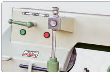
Adjustable cutting feed control valve
