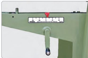
Adjustable cutting pressure regulator (Spring tension)
