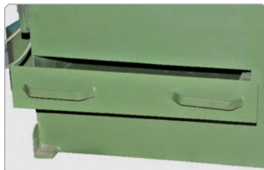
Chip collecting tray for easy cleaning
