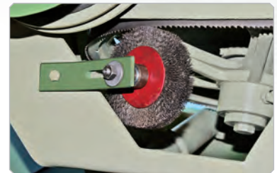
Chip removing wire brush assembly for longer blade life
