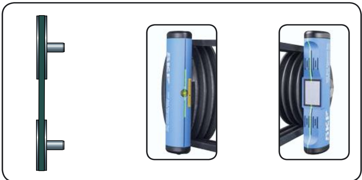
Figure 9: Pulleys perfectly aligned
