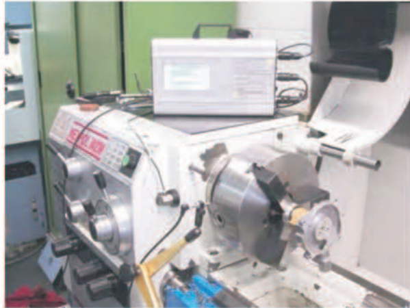
Processing of electric motor housing
