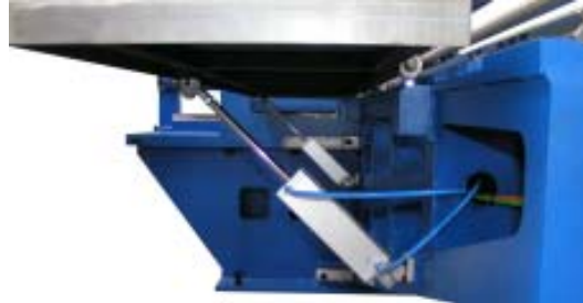
tilting table with two pneumatic cylinders
