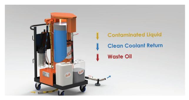
The Tramp Oil Separator is able to effectively separate tramp oils, and is especially suited to the regeneration of water-mixed coolants. Compact and mobile, it is easy to manouver and is ideal for use on individually filled machine tools and machining centres, with a capacity of 70 litres.
