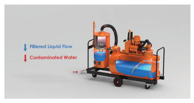
The Mark V is our largest manually manouvered Freddy. Available in 310 or 500 litre models, it has a tilting filter tank, enabling quick and easy emptying of the 60 litre basket. It comes with a complete tool kit and a 200um filter bag as standard. With the ability to vacuum at 270 litres per minute and return at 130 litres per minute the Mark V can empty, filter and return coolant to a machine tool sump in minutes.
