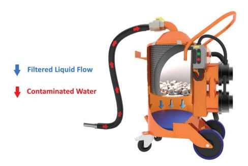
Like the Micro, the Micro Plus has a 50 litre tank capacity and a 37 litre perforated steel filter basket. It comes with a 38mm or 51mm hose and a 200um filter bag as standard. With the ability to vacuum 238ltr per minute, and air flow of 3000 litre per minute, it enjoys all the benefits of the standard Micro but with now the ability to empty under pressure in just 45 seconds.
