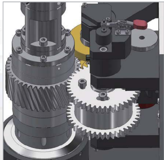
4-Station Ring Loader & Chamfering/Deburring Device
