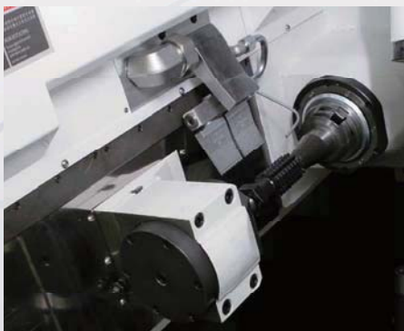
High pressure air nozzle & Coolant nozzle
