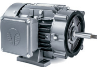
GR3 NEMA Premium 56J Pump Motor Series • 1/3 - 3HP • 2/ 4/ 6 극 • 56J - 56HJ • TEFC • 300 Series SS Shaft
