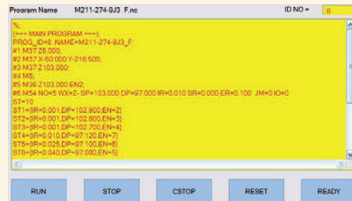
Step2 : Automatically generate a program for discharging
