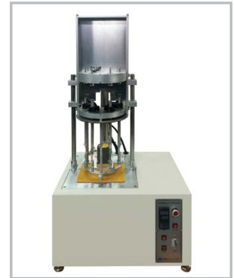
저온(견만)시험기 Low Temperature Testing of Rubber (Gehman)
