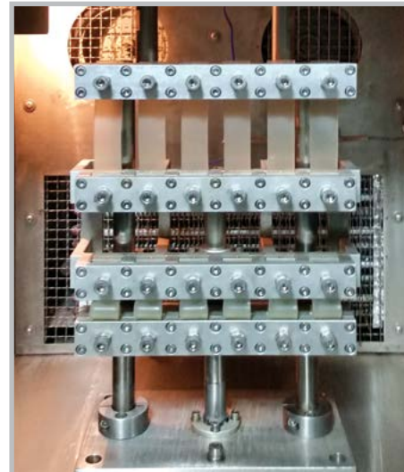
챔버형 굴곡시험기 DeMattia Chamber Type Flex Tester (Low to high temp.)
